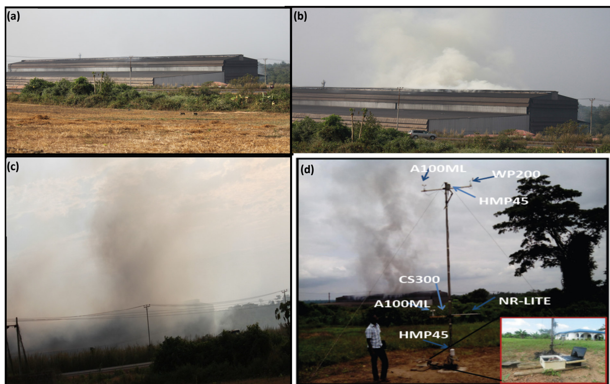
Fig. 3: Plume release scenario (a) idle period; (b) commencement of operation; (c) peak of smelting operation; and (d) during the field measurement; at the scrap-iron recycling plant located at Fashina, Ile-Ife, Ife Central Local Government Area, Southwestern Nigeria.
